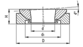
$\begin{array}{ll} D & = 70 \\ d & = 36 \\ d1 & = 48 \\ H & = 20 \\ Max \ screw \ dimension = M30 \\ Static \ load \ (kN) & = 330 \\ Weight \ (g) & = 372 \\ \end{array}$
